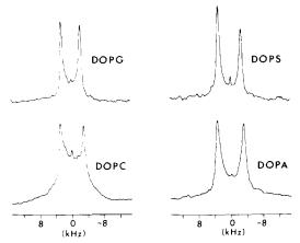
Fig. 3. 30.7 MHz<sup>2</sup>H-NMR spectra of fully hydrated [C<sub>11</sub>-<sup>2</sup>H<sub>2</sub>]DOPC, [C<sub>11</sub>-<sup>2</sup>H<sub>2</sub>]DOPG, [C<sub>11</sub>-<sup>2</sup>H<sub>2</sub>]DOPA, [C<sub>11</sub>-<sup>2</sup>H<sub>2</sub>]DOPS. Sample preparation and the conditions for obtaining the <sup>2</sup>H-NMR spectra are identical to those described in the legend of Fig. 2.
